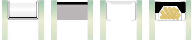
Duralite™ 0.30 U-Factor Super Spacer® 0.31 U-Factor Intercept® 0.32 U-Factor Aluminum Spacer 0.34 U-Factor
